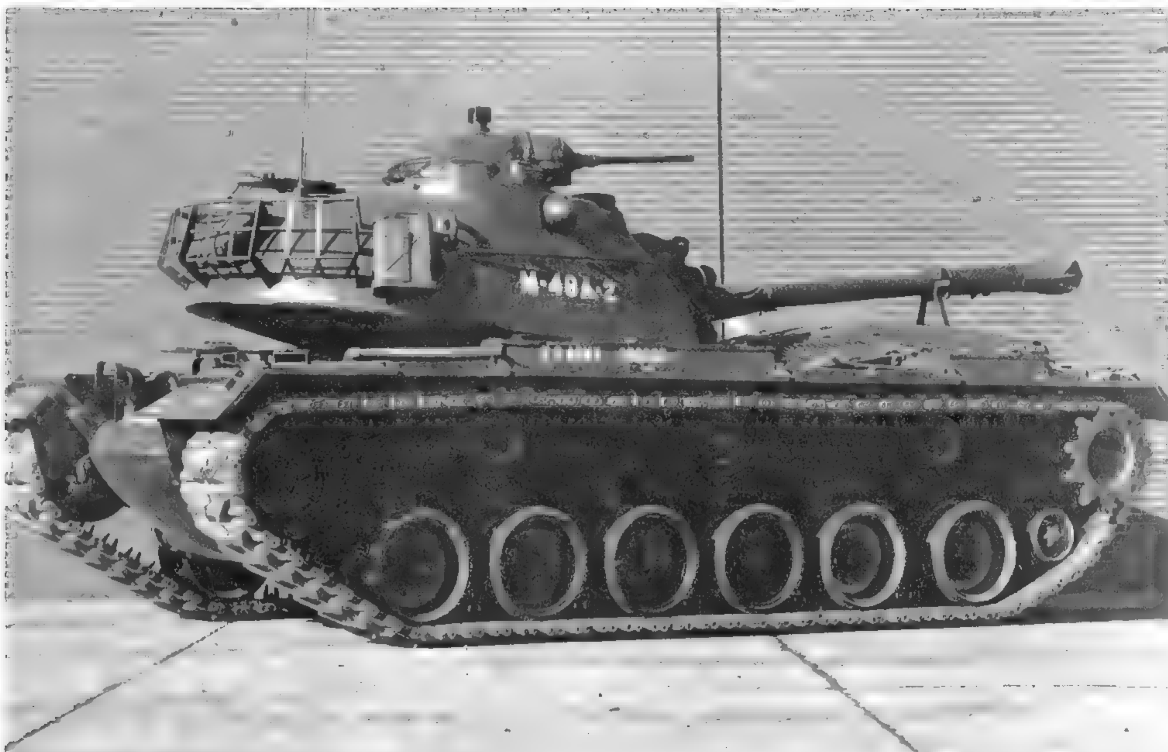
The M48A2 had an elliptical-shaped front hull. On the rear of the turret is the stowage rack added starting with the M48A1. (Photo courtesy of the Patton Museum)
